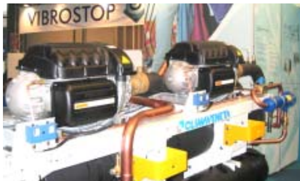
Two Turbocor compressors mounted on Climaveneta chiller
