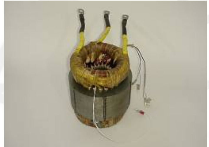
120kW motor the same size as a 0.75kW motor
